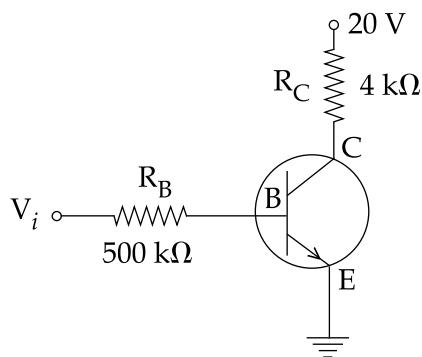
In the circuit shown in the figure, the input voltage  $V_i$  is 20 V,  $V_{BE} = 0$  V and  $V_{CE} = 0$  V, what are the values of  $I_B$ ,  $I_C$  and  $\beta$  ?
