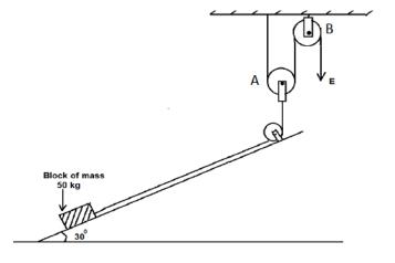
56) Refer to figure in question 55. Pulleys in the figure are massless and frictionless. Neglecting friction between block and the ramp, the force that should be applied vertically downwards, at E, to slide the block along the ramp without acceleration is (g=10 m·s<sup>-1</sup>)
